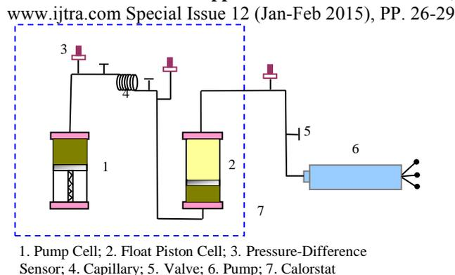
1. Pump Cell; 2. Float Piston Cell; 3. Pressure-Difference Sensor; 4. Capillary; 5. Valve; 6. Pump; 7. Calorstat
