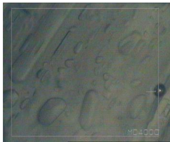
Fig.5 Etchpit pattern of TTCS crystal with water in 10 s
