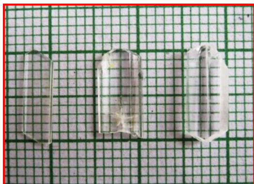
Fig.1 Grown TTCS crystal by slow evaporation method
