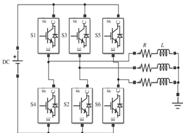
Fig.1: three-phase voltage source pwm Inverter
