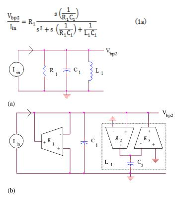
Fig. 2(a) Passive transimpedance band-pass biquad (b) OTA-C transimpedance band-pass biquad derived from (a)
