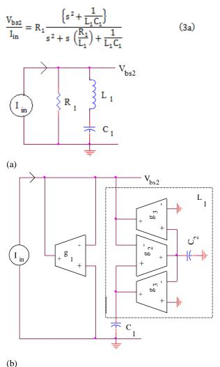
Fig. 4(a) Passive transimpedance band-stop biquad (b) OTA-C transimpedance band-stop biquad derived from (a)
