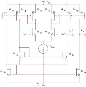
Figure 6: Schematic circuit of CMOS DO-OTA
