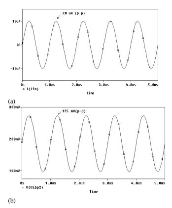
Fig. 11. Transient analysis: input and output waveforms of the OTA based Transimpedance-mode Inverse Band-pass Biquad of Fig. 3(b)
