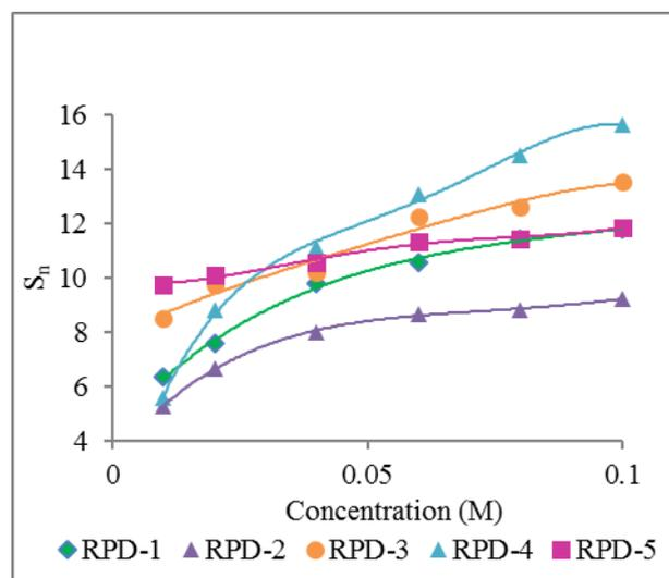
**Figure 5: Variation of solvation number ( $S_n$ ) with concentration of phenyl pyrimidine derivatives in 1,4-dioxane at 298.15 K.**
