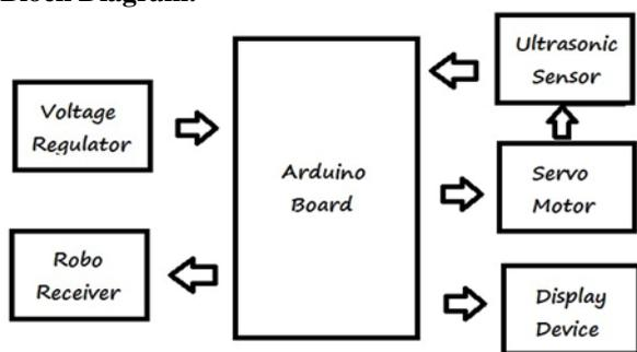
Figure 1.1 Block Diagram
