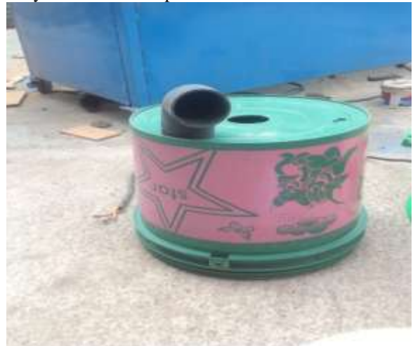
Figure 1: Top part of Dust Collector
