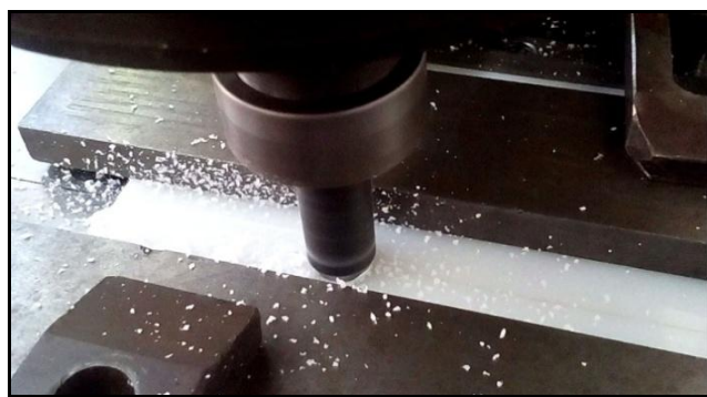
Fig. 12: High rotation speed caused ejection of polymer
