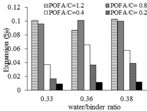
Fig. 2. Expansion of ECC bars due to ASR at age of 30 days with different w/b and POFA/C ratios.
