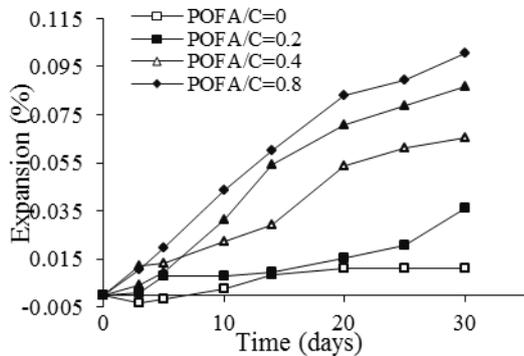
Fig. 4. Effect of POFA/C ratio on the expansion of ECC bars due to ASR at w/b=0.36.
