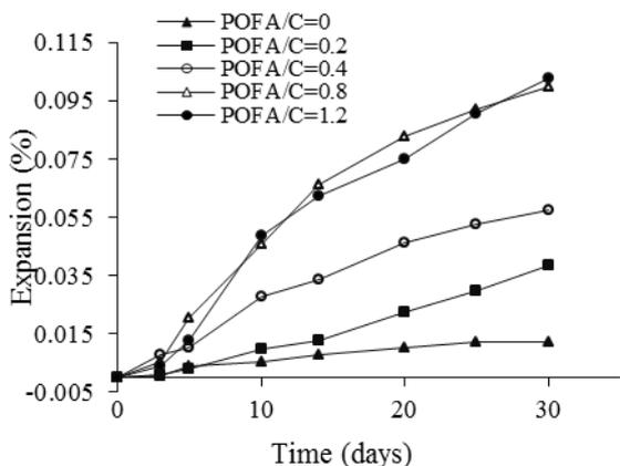
Fig. 5. Effect of POFA/C ratio on the expansion of ECC bars due to ASR at w/b=0.38.
