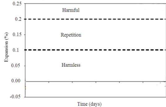
**Fig. 1. Classification ranges of length change stipulated by ASTM C1260.**
