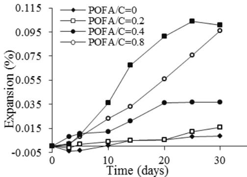
Fig. 3. Effect of POFA/C ratio on the expansion of ECC bars due to ASR at w/b=0.33.
