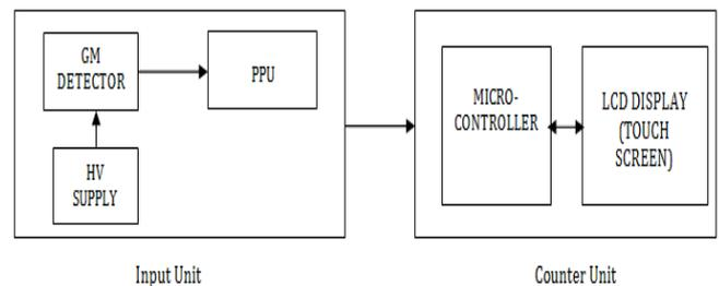
Fig 2 Block Diagram of Level gauge
