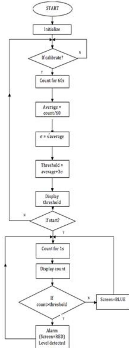
Fig 4 flow chart giving programming logic
