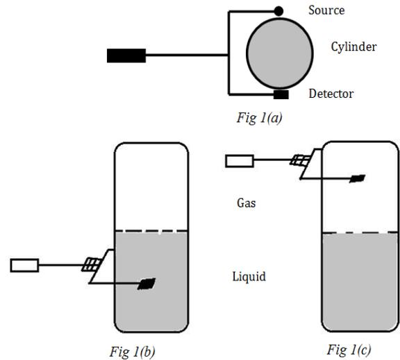
Fig 1 source detector arrangement of Level gauge
