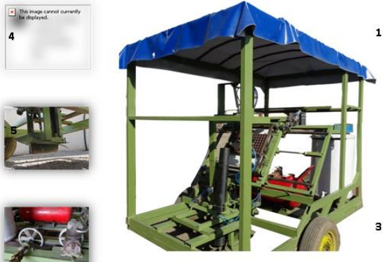
Fig.1. Constructed transpalnter and components(1: ratchet mechanism 2: furrower 3: air reservoir and compressor 4: PLC and control box 5: pick up arm 6: x-direction displacement mechanism)
