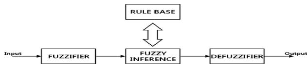
Fig. 4. General configuration of fuzzy logic controller
