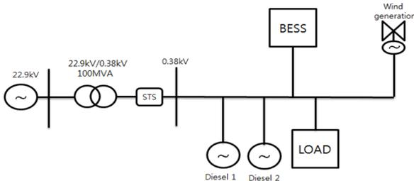
Fig. 11. Microgrid test model
