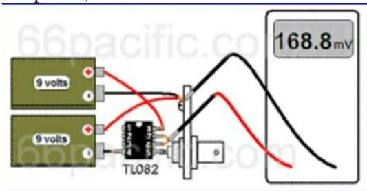
Above shows the physical layout of the meter a digital voltmeter is connected to ground and pin.6 and 7 of the op-amp which are shorted together . In this circuit the pins.1,2,3 of the IC are not used.
