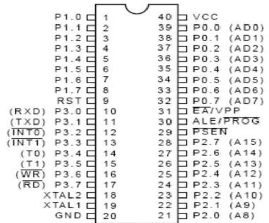
PIN DIAGRAM OF AT89C51
