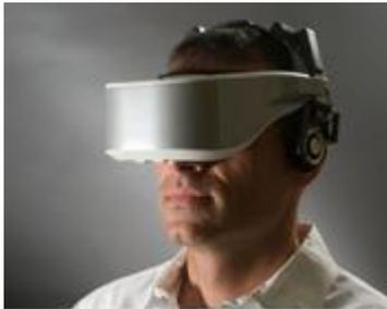
Figure 2: A head mounted display
