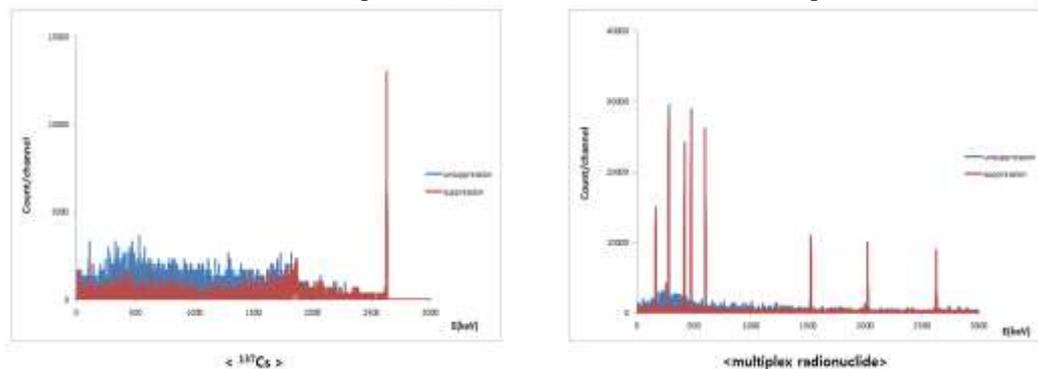
Fig. 5. The un-suppressed and suppressed spectrum by  $^{137}\text{Cs}$  and multiplex radionuclide source
