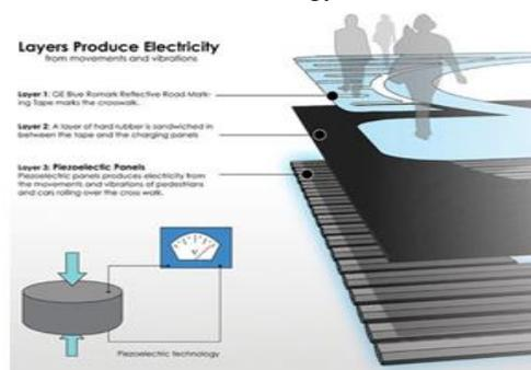
Fig 2 : Illustration of Layers of Piezoelectric Material
