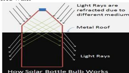
FIG 7 : ILLUSTRATION OF WORKING OF SOLAR BOTTLE BULB
