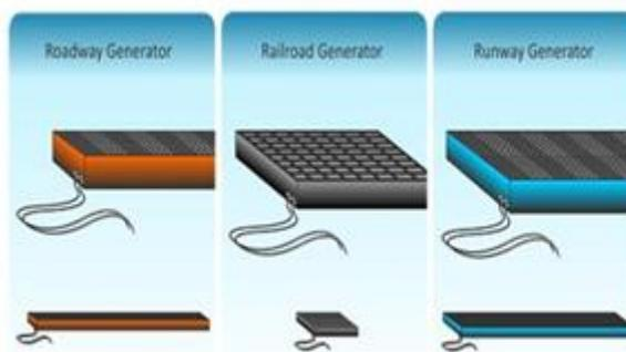
Fig 4 : Various kinds of Piezoelectric Generators
