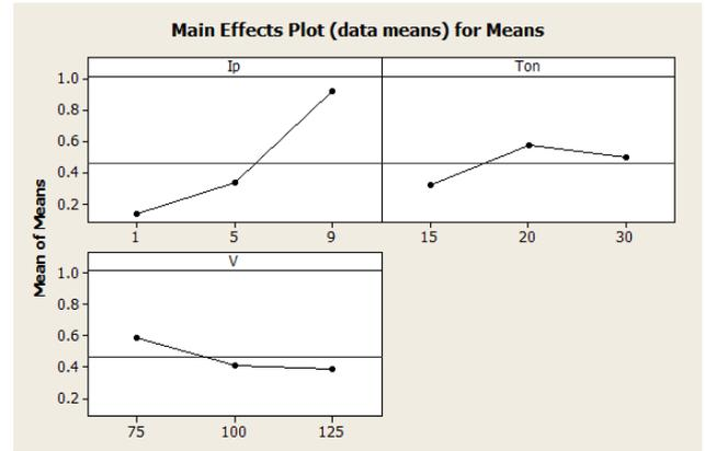
Figure 1: Main Effect Plot For Means For MRR
