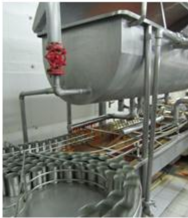
Fig. 4. The used in-line gravity sauce filling equipment
