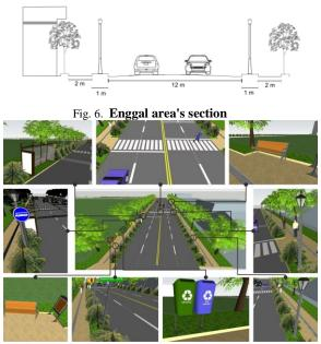
Fig. 7. Enggal area's pedestrian ways re-arrangement design
