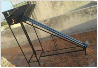
On this side, there are two holes for fitting tubes. For tightening and leak-proof of tubes, rubber ring are provided.
