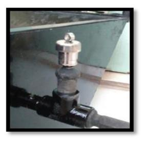
Safety valve use for the safety of the glass material of the system. Because the top side of insulation box is made with plane glass plate and also insulation box is assembled with the evacuated tubes.
