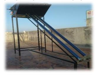
And also valves and T-section piping joint are provided on the adjacent of inclined plane for pouring water inside and extracting the hot water outside. And both boxes are assembled together and between them glass wool is provided for heating resisting purpose (Maintain inside temperature). Now, to make stand as per specification, no. of L-section channel are stick together by welding process. And last, the upper cover which is made with double glass and wooden frame is fixing with tightly.
