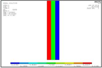
Fig. 6 Hoop's stress pattern for case study of Ammonia Converter
