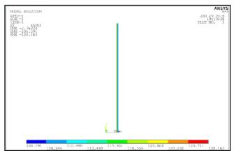
Fig.4 Hoop's stress pattern for Mono Wall Pressure Vessel
