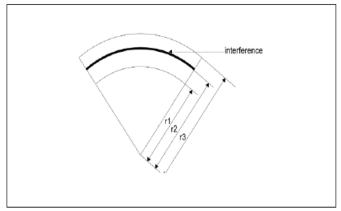
Fig.2 Portion of c/s of Multi Wall Vessel with interference
