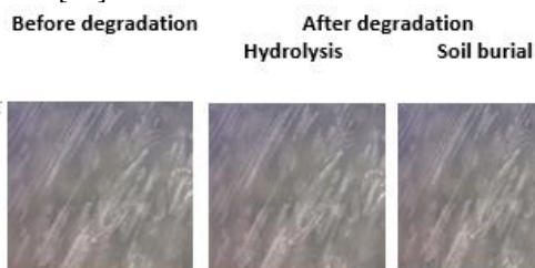
Fig.12: The surface morphology for pure Polypropylene before and after degradation for 3 month (200X).
