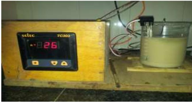
**Fig 3: Experimental Setup for Starch Isolation with PID Controller**
