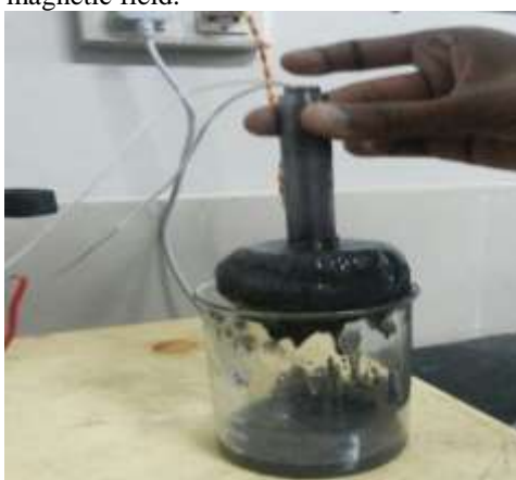
Fig. 3(b) Actual schematic of MR fluid after applying magnetic field
