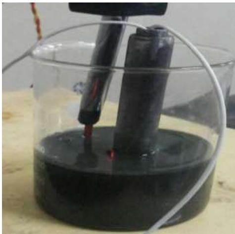
Fig. 2(b) Actual schematic of MR fluid before applying magnetic field
