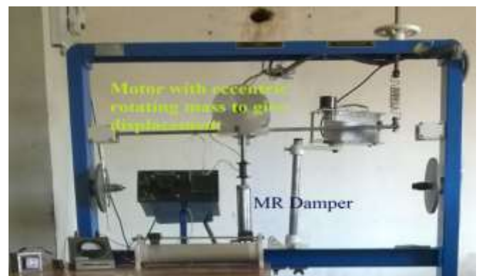
Fig.8 Experimental setup for MR damper testing
