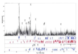
Fig.6 (a) XRD pattern of Bagasse ash at 1200°C for 3h
