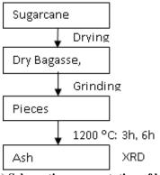
Fig. 5(a) Schematic representation of bagasse ash
