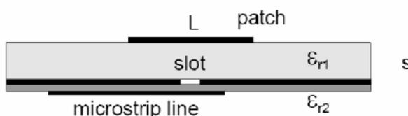
**Figure 5: Aperture couple feed for Microstrip Patch**
