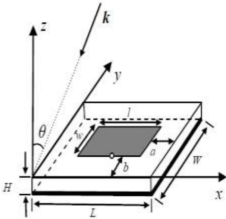
**Figure 3: Structure of Microstrip Patch Antenna**
