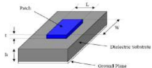
Figure 2: Microstrip Patch Antenna Top View.
