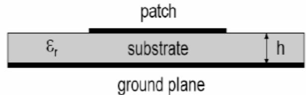
Figure 1: Microstrip Patch Antenna front view.
