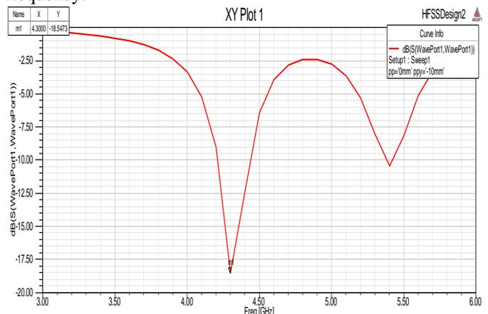
**Figure 6: Simulation of S11 Parameter (Return Loss)**
