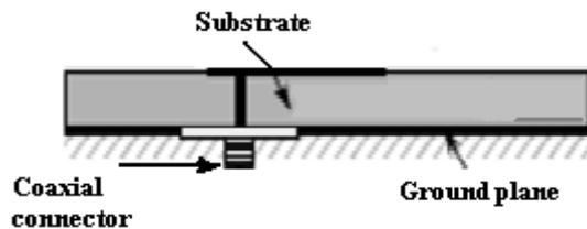
**Figure 4: Probe Feed for Microstrip Patch.**
