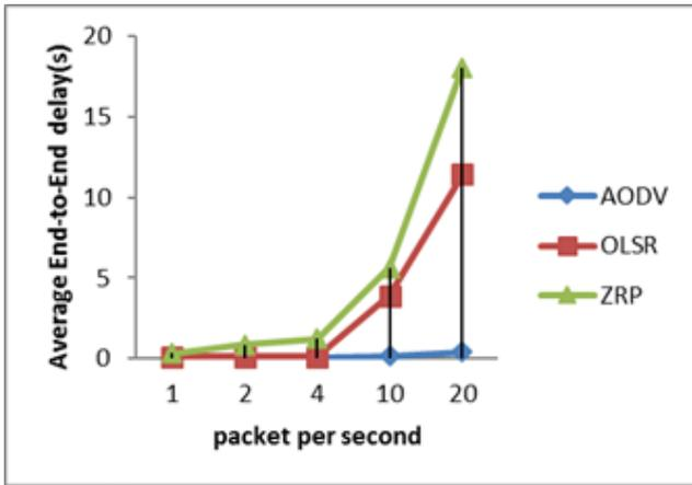
Figure 3: Average End-To-end Delay Vs Packet Per second
