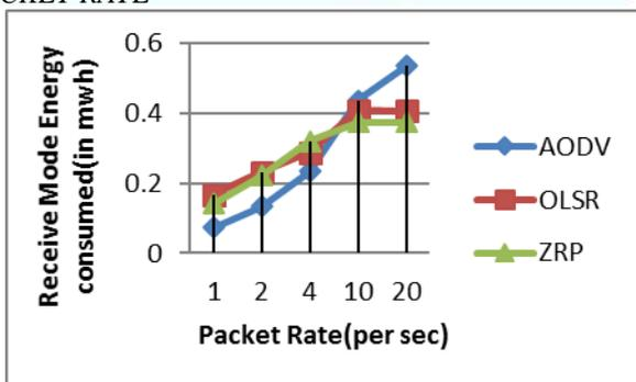
Figure 11: Receive mode energy consumed Vs Packet rate
