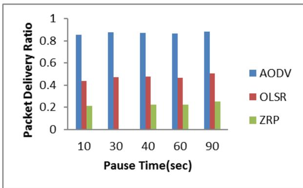
Figure 9: Packet Delivery ratio (PDR) Vs Pause time
