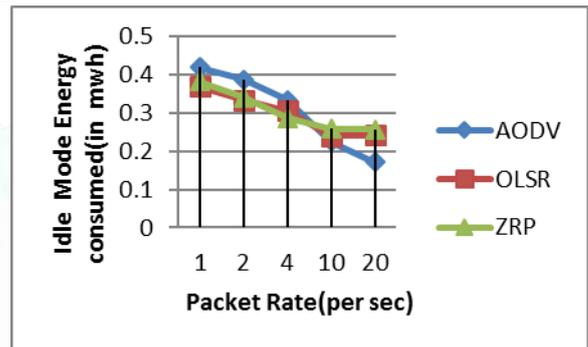
Figure 12: Idle mode energy consumed Vs Packet Rate
