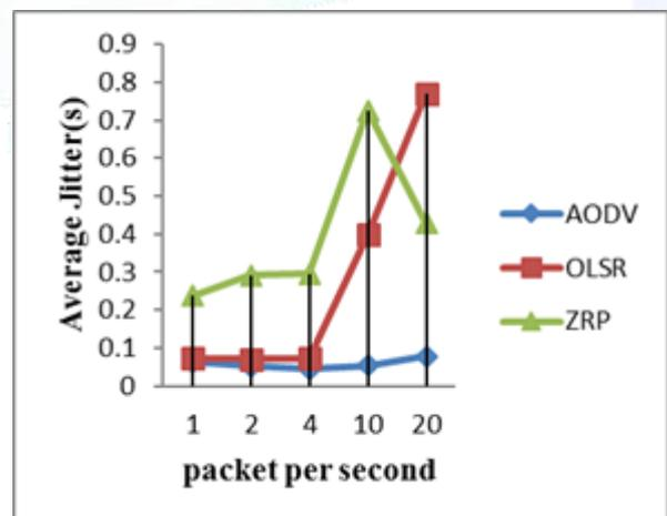
Figure 2: Average Jitter Vs Packet per Second
