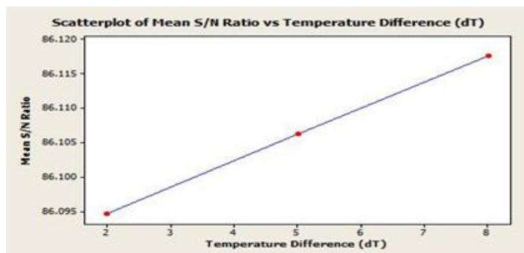
Fig 2: variation of mean of S/N ratio with temperature difference.
