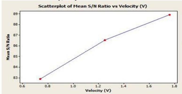
Fig 1: variation of mean of S/N ratio with air velocity.
