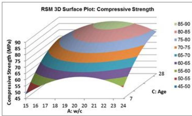
Figure (19): Three dimension RSM maximum compressive response surfaces for moist cured RPC between w/c and age.
