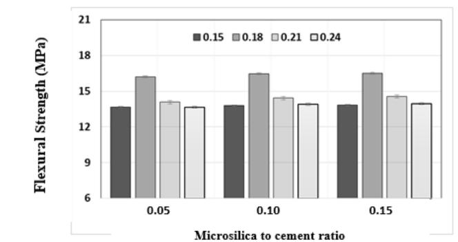
Figure (18): Flexural strength results at 28-day for autoclave cured specimens
