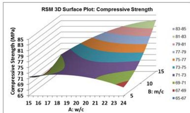
Figure (26): Three dimension RSM maximum compressive response surfaces for autoclaved cured RPC between w/c and m/c.
