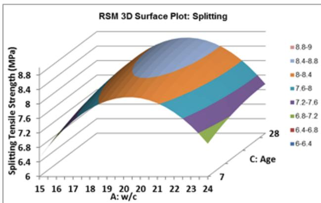
Figure (21): Three dimension RSM maximum splitting response surfaces for moist cured RPC between w/c and age.
