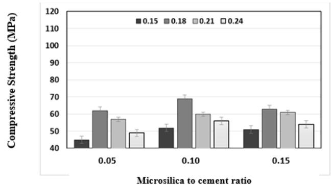
Figure (1): Compressive strength results at 7-day for moist cured specimens
