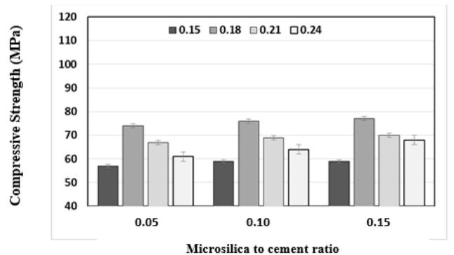
Figure (2): Compressive strength results at 14-day for moist cured specimens
