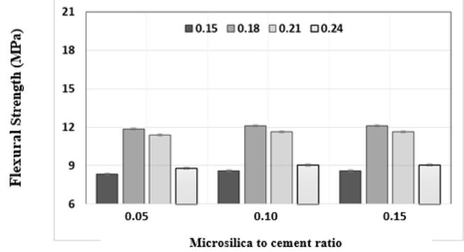
Figure (15): Flexural strength results at 28-day for moist cured specimens.
