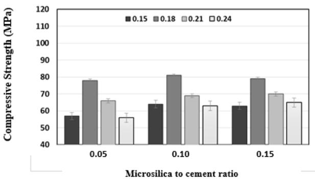
Figure (4): Compressive strength results at 7-day for autoclave cured specimens.
