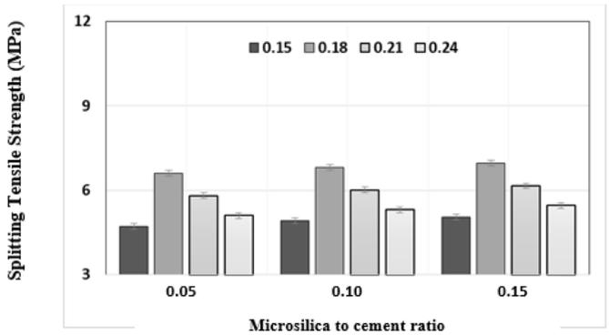
Figure (9): Splitting tensile strength results at 28-day for moist cured specimens.
