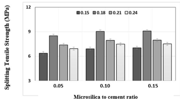
Figure (10): Splitting tensile strength results at 7-day for autoclave cured specimens.
