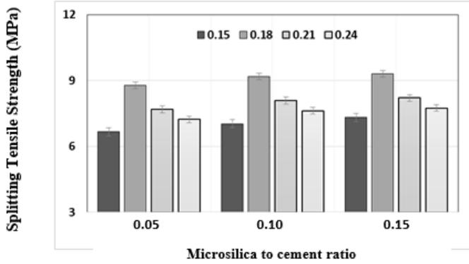
Figure (11): Splitting tensile strength results at 14-day for autoclave cured specimens.
