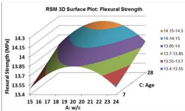
Figure (29): Three dimension RSM maximum flexural response surfaces for autoclaved cured RPC between w/c and age.
