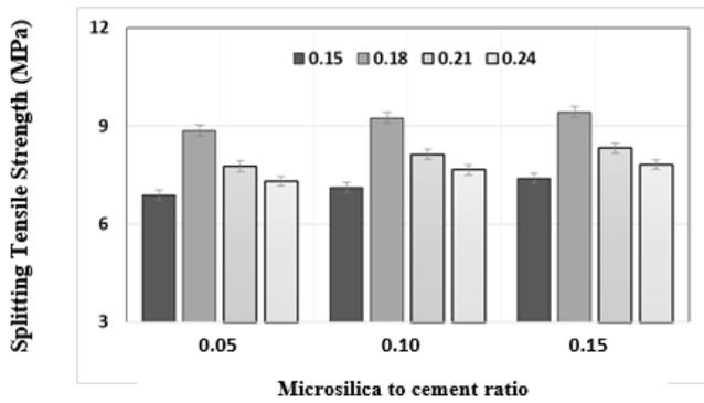
Figure (12): Splitting tensile strength results at 28-day for autoclave cured specimens
