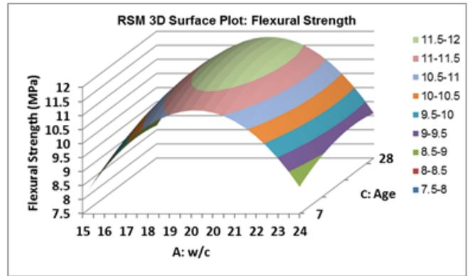
Figure (23): Three dimension RSM maximum flexural response surfaces for moist cured RPC between w/c and age.
