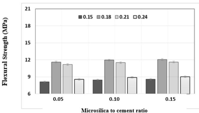
Figure (14): Flexural strength results at 14-day for moist cured specimens.
