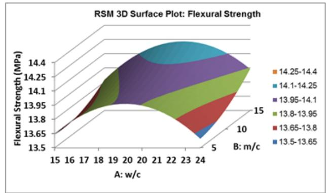
Figure (30): Three dimension RSM maximum flexural response surfaces for autoclaved cured RPC between w/c and m/c.
