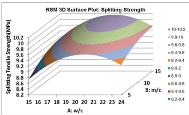
Figure (28): Three dimension RSM maximum splitting response surfaces for autoclaved cured RPC between w/c and m/c.
