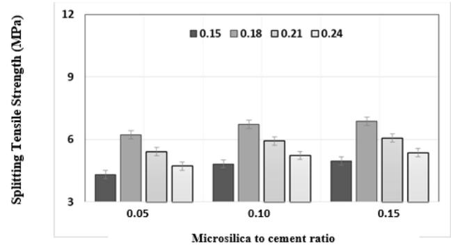
Figure (8): Splitting tensile strength results at 14-day for moist cured specimens.
