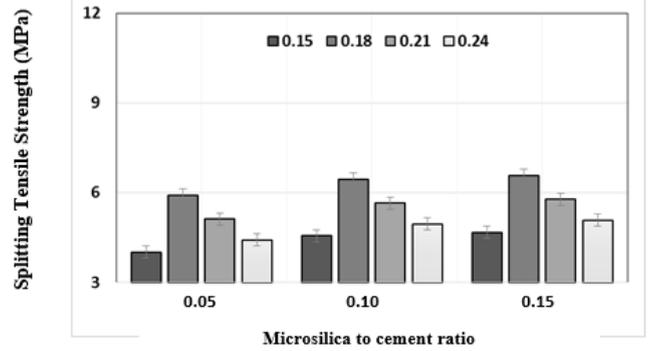
Figure (7): Splitting tensile strength results at 7-day for moist cured specimens.
