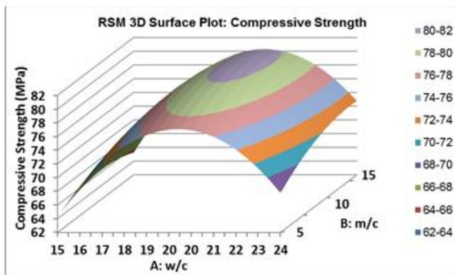
Figure (20): Three dimension RSM maximum compressive response surfaces for moist cured RPC between w/c and m/c.
