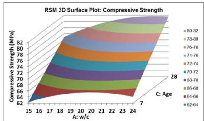
Figure (25): Three dimension RSM maximum compressive response surfaces for autoclaved cured RPC between w/c and age.
