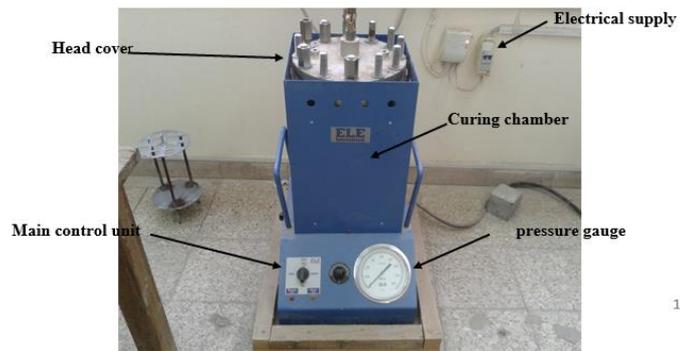
Plate 1: Autoclave curing apparatus in the University of Technology/Baghdad
