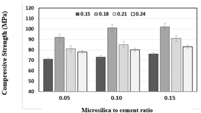
Figure (6): Compressive strength results at 28-day for autoclave cured specimens.
