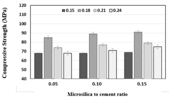
Figure (5): Compressive strength results at 14-day for autoclave cured specimens.
