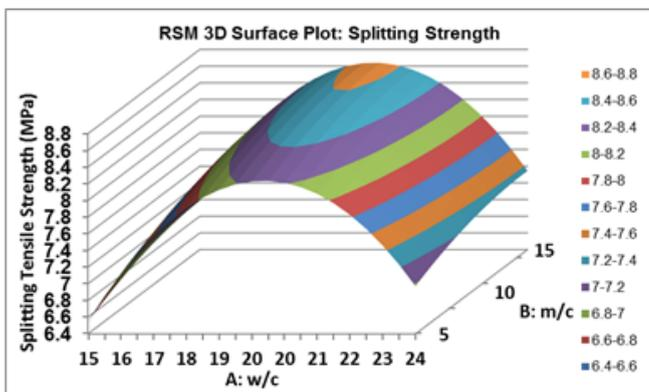
Figure (22): Three dimension RSM maximum splitting response surfaces for moist cured RPC between w/c and m/c.
