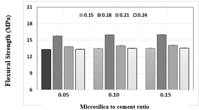
Figure (16): Flexural strength results at 7-day for autoclave cured specimens.
