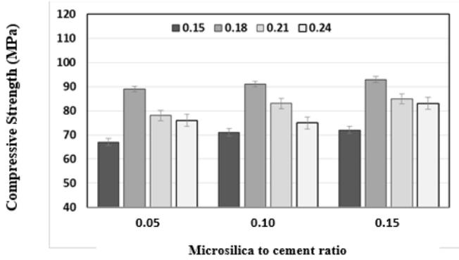
Figure (3): Compressive strength results at 28-day for moist cured specimens.
