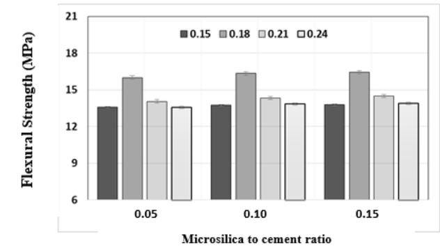
Figure (17): Flexural strength results at 14-day for autoclave cured specimens.
