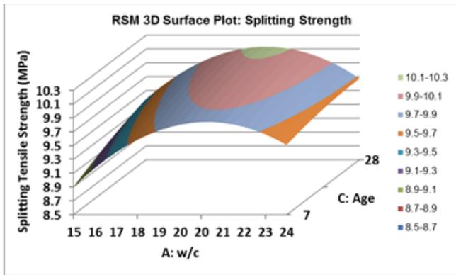
Figure (27): Three dimension RSM maximum splitting response surfaces for autoclaved cured RPC between w/c and age
