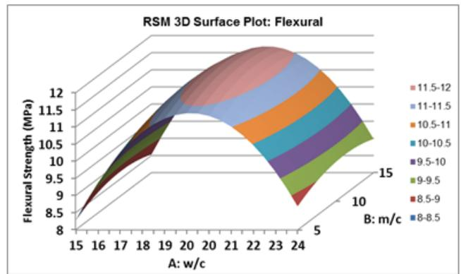
Figure (24): Three dimension RSM maximum flexural response surfaces for moist cured RPC between w/c and m/c.
