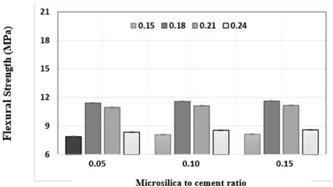
Figure (13): Flexural strength results at 7-day for moist cured specimens
