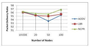
Fig. 2. Packet Delivery Ratio Vs Number of Nodes(nodes are static)
