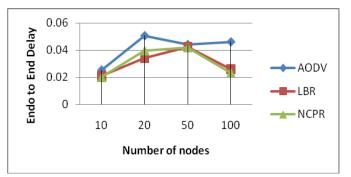
Fig. 3. End to End Delay Vs Number of Nodes (nodes are static)
