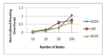
Fig. 4. Normalized Routing Overhead Vs Number of Nodes(nodes are dynamic)
