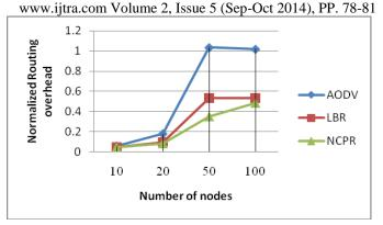
Fig. 1. Normalized Routing Overhead Vs Number of Nodes (nodes are static)
