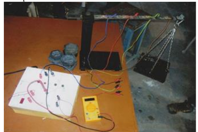
Fig. 1 Experimental Setup for measurement of stress
