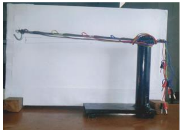
Fig. 2 Experimental Setup for measurement of deflection
