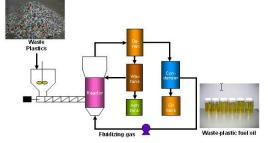
Process of Pyrolysis of Waste Plastics Technology Fig2. Process of pyrolysis of waste plastic
