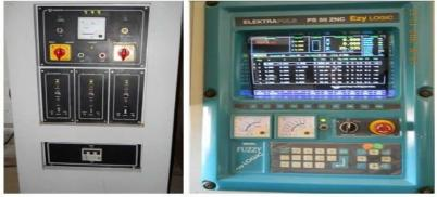
Figure 3.2 Control unit of EDM machine
