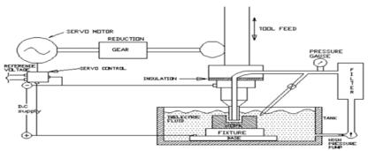
Figure 1. 1 Set up of Electric discharge machining
