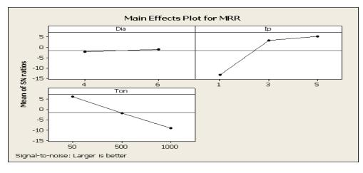
Figure 4.1 Main effect plot for S/N ratios (MRR)
