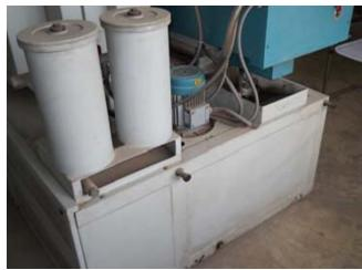
Figure 3.1 Dielectric reservoir 2) *Power generator and control unit* –
