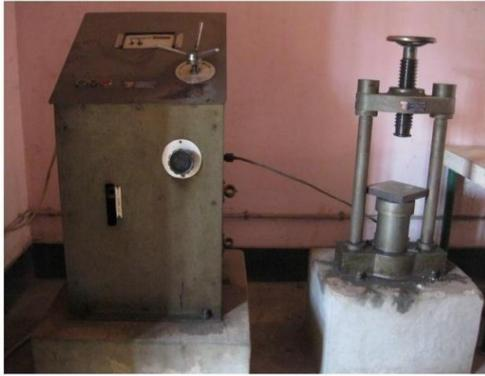
Fig 3.3: Cold Uniaxial Pressing Machine
