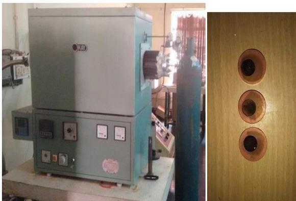
Fig. 3.4: Horizontal Tubular Furnace Fig. 3.5: Samples after sintering
