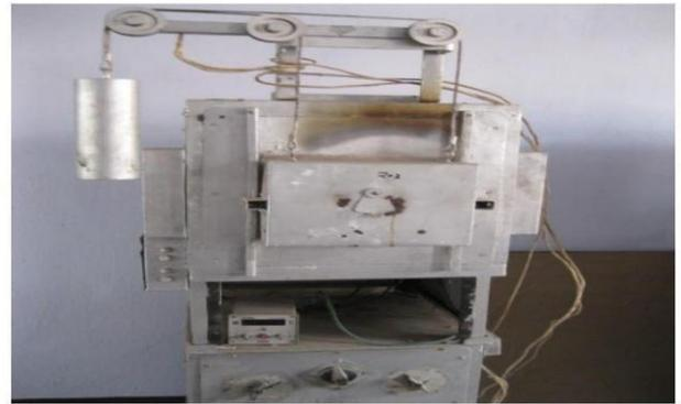
Fig. 3.6: Heat Treatment Furnace
