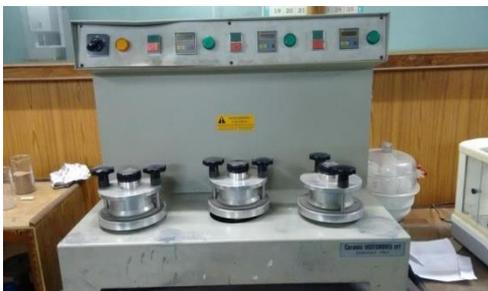
Fig 3.1: Ball Planetary Mill
