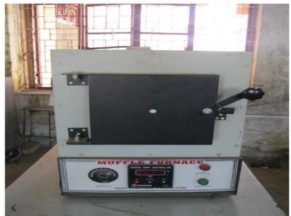
Fig. 3.7: Closed Muffle Furnace
