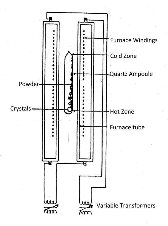
Fig 1 : Schematic view of the furnace showing the position of ampoule inside the two zone furnace during crystal growth.
