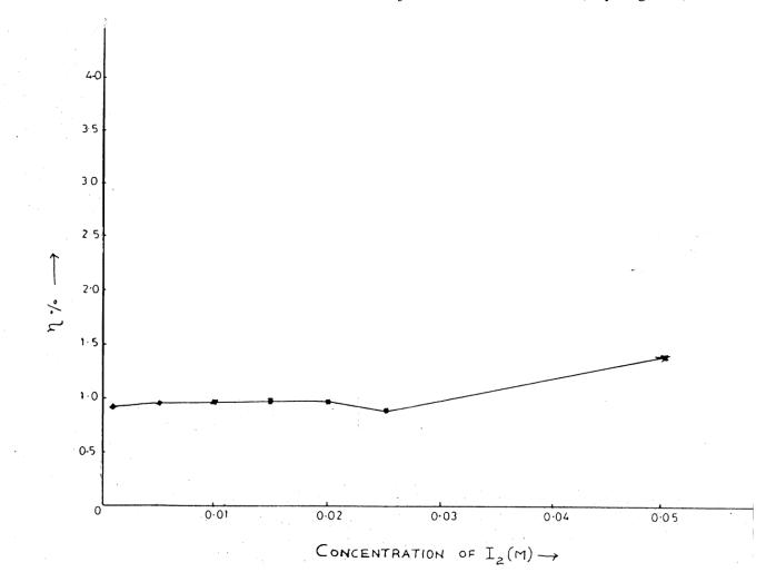
Fig 3: Plot of efficiency versus iodine concentrations I2(M) for PEC solar cells based on MoTe2.
