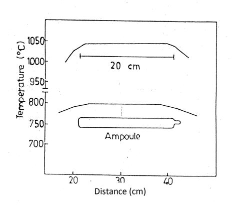
Fig 2: Temperature profile of the furnace.
