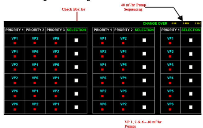
Fig 11 : Vacuum Pump Priority Selection in Casting
