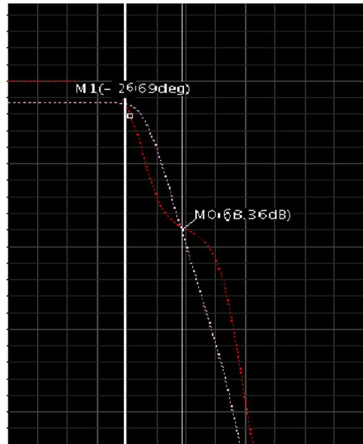
Figure 9 .phase and gain margin of Op-Amp
