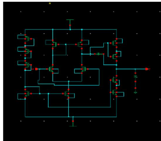
Figure.3 The proposed CMOS Op-Amp circuit
