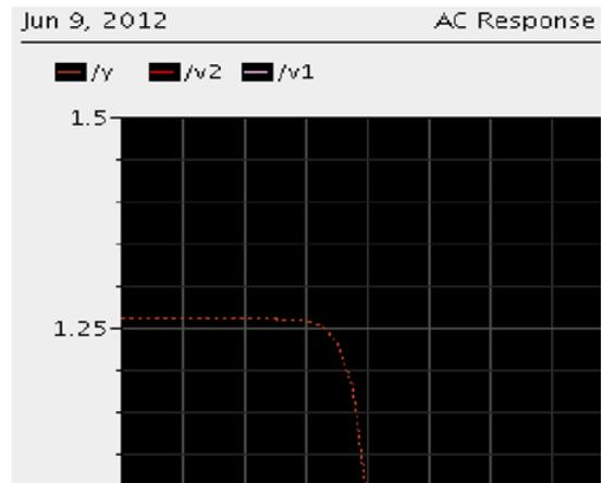
Figure 4. Frequency Response Plot with  $C_L=10$  pf
