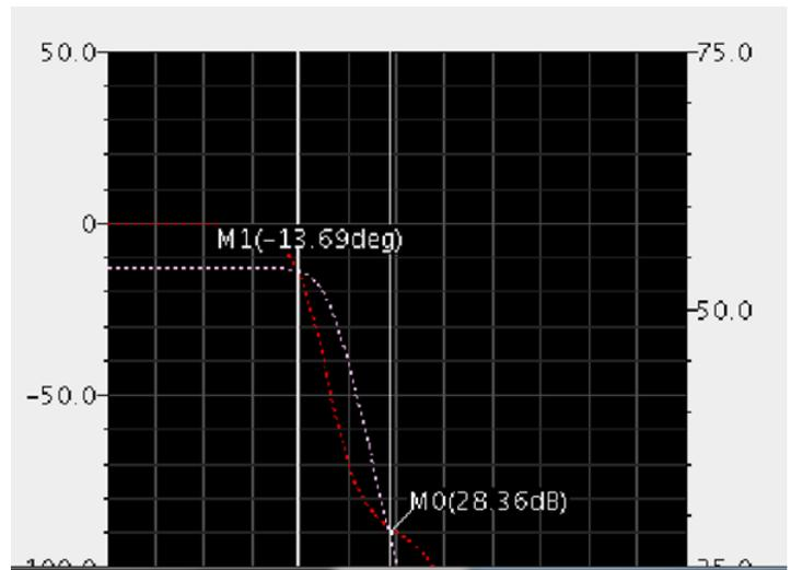
Figure 8 .phase and gain margin of Op-Amp
