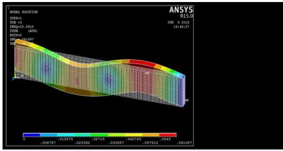
Fig. 3. Mode shape 3 of undamaged beam
