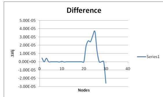
Fig. 9. Difference in curvature mode shape 3
