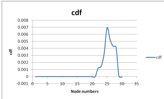
Fig. 10. Curvature damage factor for last loading condition
