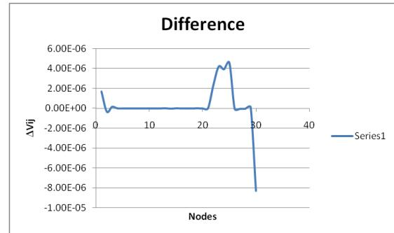
Fig. 7. Difference in curvature mode shape 1
