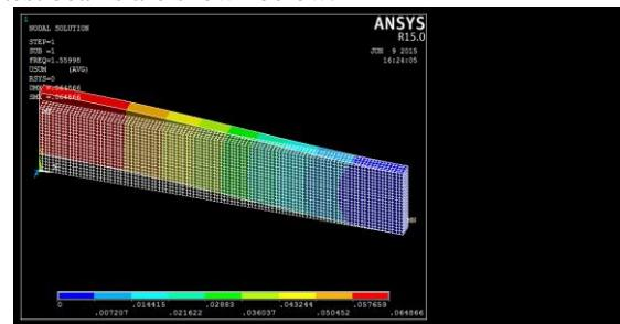
Fig. 1. Mode shape 1 of undamaged beam
