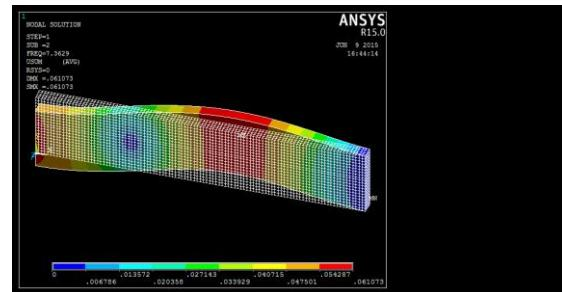
Fig. 2. Mode shape 2 of undamaged beam
