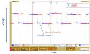
Fig. 15 Encoder feedback signal
