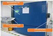
Fig. 10 HALT temperature test chamber
