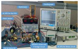
Fig. 9 Hardware setup
