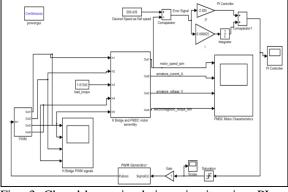
Fig. 3 Closed-loop simulation circuit using PI controller
