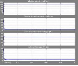
Fig. 6 Motor characteristics with PI controller
