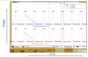
Fig. 14 PWM pulsed signals of low-side MOSFETs
