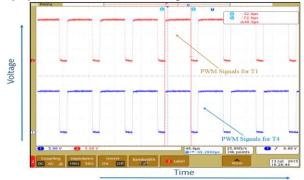
Fig. 13 PWM pulsed signals of high-side MOSFETs
