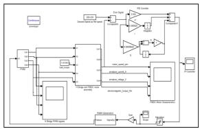
Fig. 4 Closed-loop simulation circuit using PID controller
