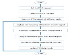
Fig. 8 Flowchart for the closed-loop control
