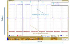
Fig. 12 PWM pulsed signals at PIC IC pins
