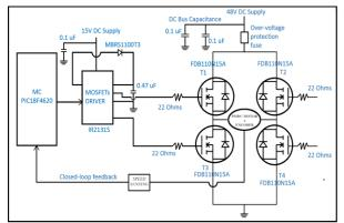
Fig. 2 Schematic diagram of the system
