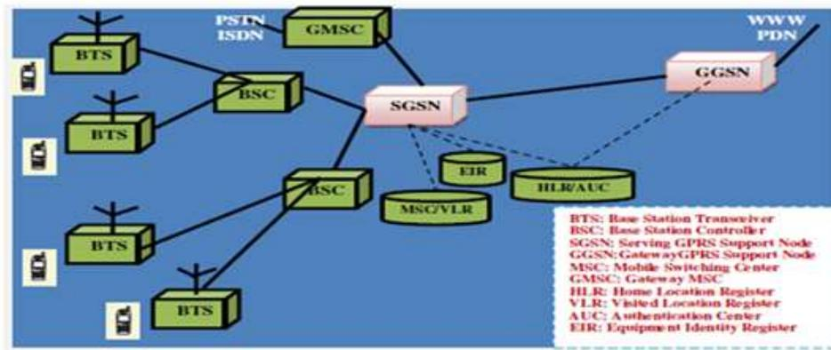
**Fig.4: General GPRS Network Architecture.**
