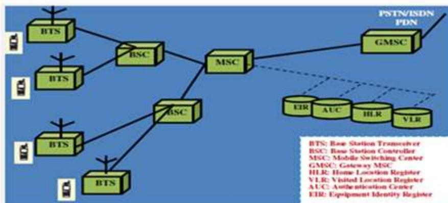
Fig.3: General GSM Network Architecture.
