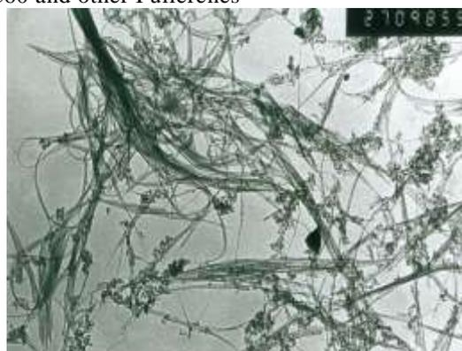
Fig. 1 Carbon single walled nano tubes (after ref.15)
