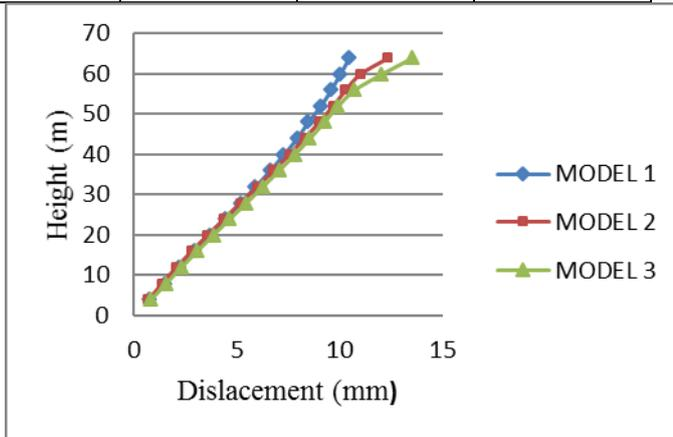
Fig.3. Variation of story displacement with respect to story height in static analysis
