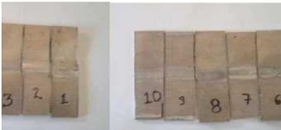
Figure 4 - a) Welded specimen performed with welding speed 3mm/s and welding current 100, 105, 110, 120 and 130A for samples numbers 1 to 5 b) welded specimen performed with welding speed 4mm/s and welding current 100, 105, 110, 120 and 130A for sample numbers 6-10, respectively
