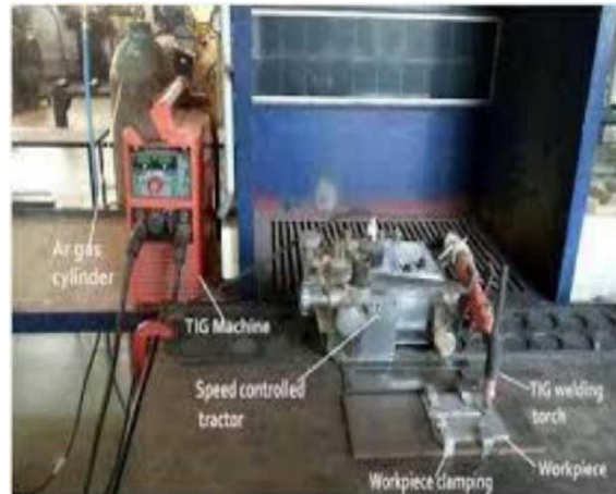
Figure 3: Automated TIG welding setup
