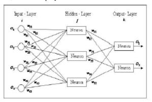
Fig.1-Layout of feed forward neural network
