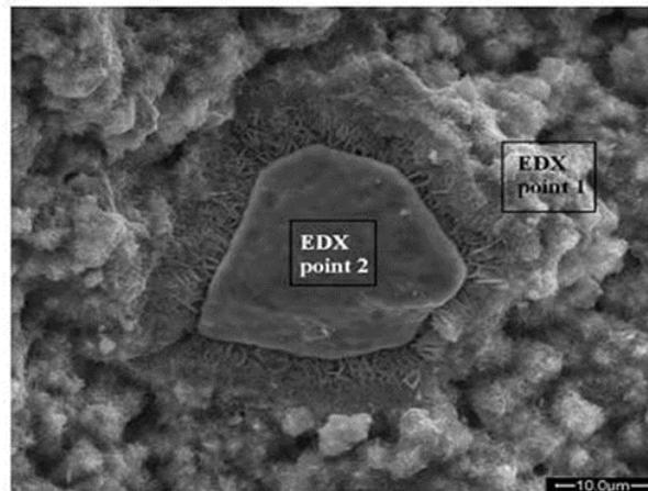
Figure 2.4 (a) SEM morphologies and EDX analysis of hydration products at the age of 28 days- SEM picture [Wang and Yan (2010)]
