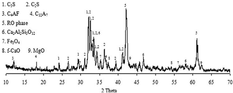
Figure 2.3. X-ray diffraction of steel slag [Wang and Yan (2010)]
