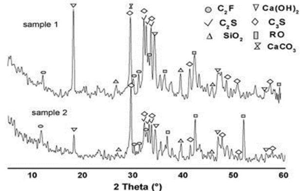
Figure 2. 2 XRD patterns of steel slag samples [Weiguo Shen., et al. (2009)]
