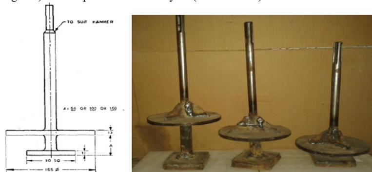
Figure 3.2. Tampers for use with a vibrating hammer for Unconfined Compressive Strength test [IS: 4332 (Part V) -1970
