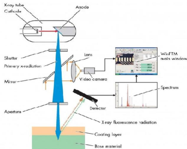
Figure 3.1 (b) XRF Instrument
