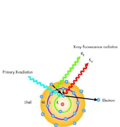
Figure 3.1 (a) Principle of XRF
