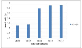
Fig 7: Effect of Solid Solvent Ratio on Starch Yield
