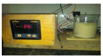
Fig 3: Experimental Setup for Starch Isolation with PID Controller
