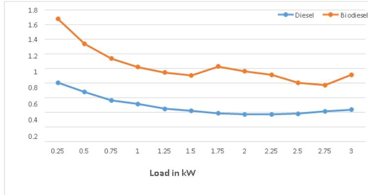
Figure 9 Graph between s.f.c. and load High Pressure and Normal Injection Timing
