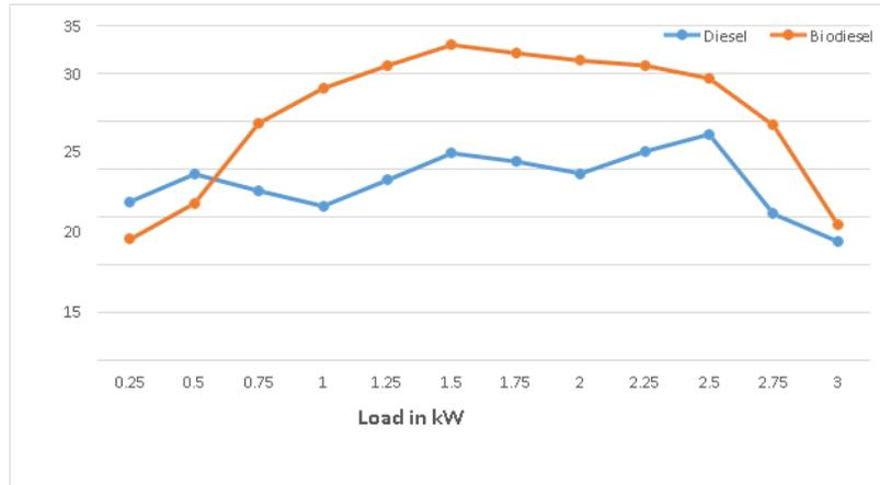
Figure 18 Graph between thermal efficiency and load
