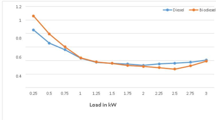
Figure 12 Graph between s.f.c. and load
