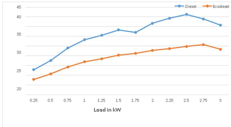
Figure 19 Graph between thermal efficiency and load High Pressure Advanced Injection Timing
