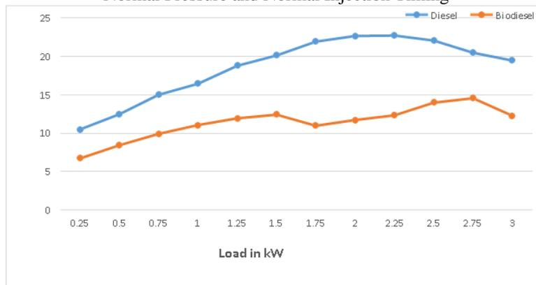
Figure 17 Graph between thermal efficiency and load High Pressure and Normal Injection Timing
