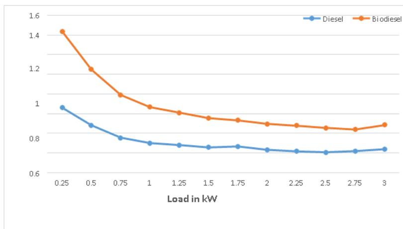
Figure 11 Graph between s.f.c. and load High Pressure and Advanced Injection Timing
