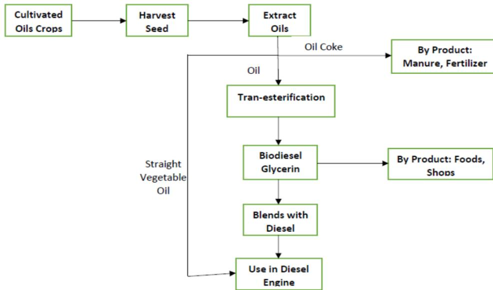
Figure 2 Schematic Diagram of Biodiesel Production.
