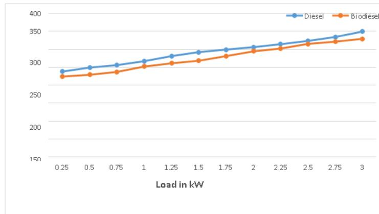
Figure 13 Graph between temperature and load High Pressure and Normal Injection Timing
