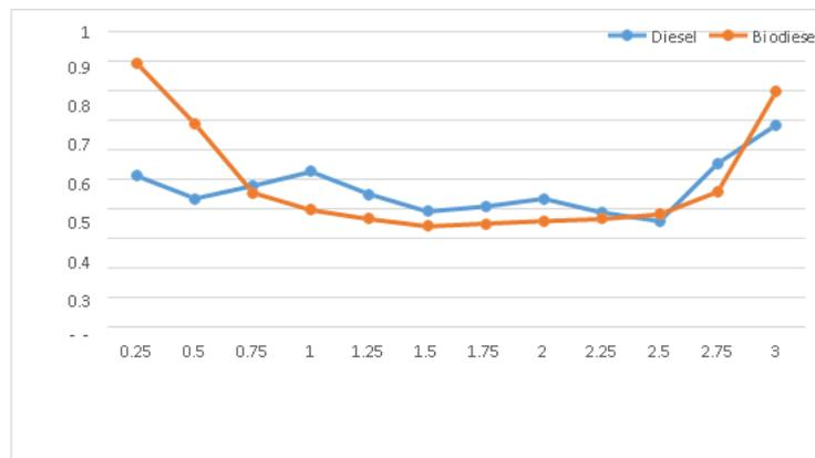
Figure 10 Graph between s.f.c and load
