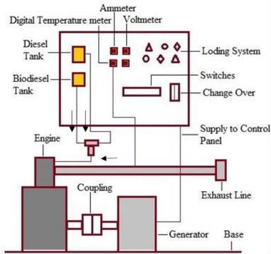
Figure 3 Schematic diagram of experiment setup
