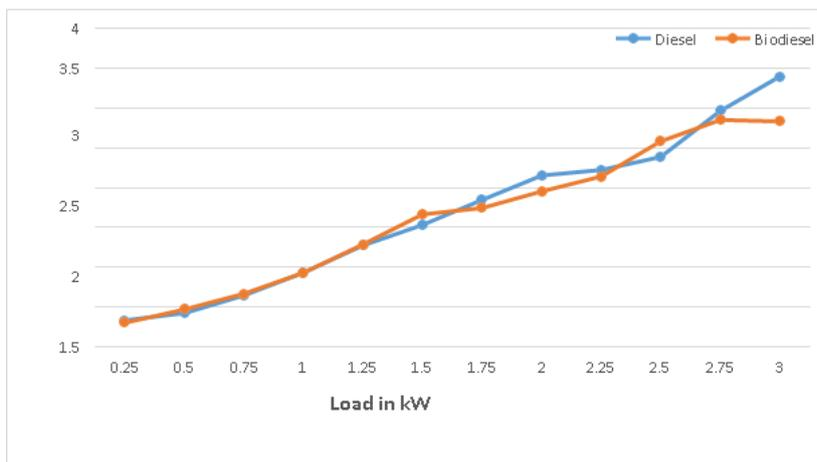
Figure 8 Graph between break power and load
