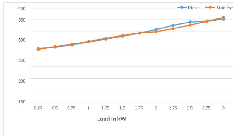
Figure 15 Graph between temperature and load High Pressure and Advanced Injection Timing
