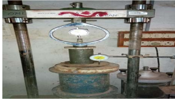
Figure 3.3 Test set up for stabilized samples.
