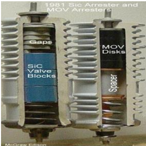
Fig(h)- Silicon Carbide Varistor and Zinc Oxide Varistor based Arrester Comparison
